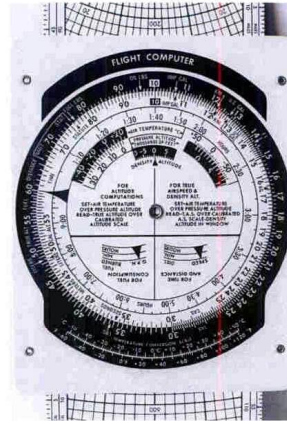
Left: Curt Andrus, '69, solved this one with just a slide rule! Above: One version of the venerable E-6B circular slide rule.
